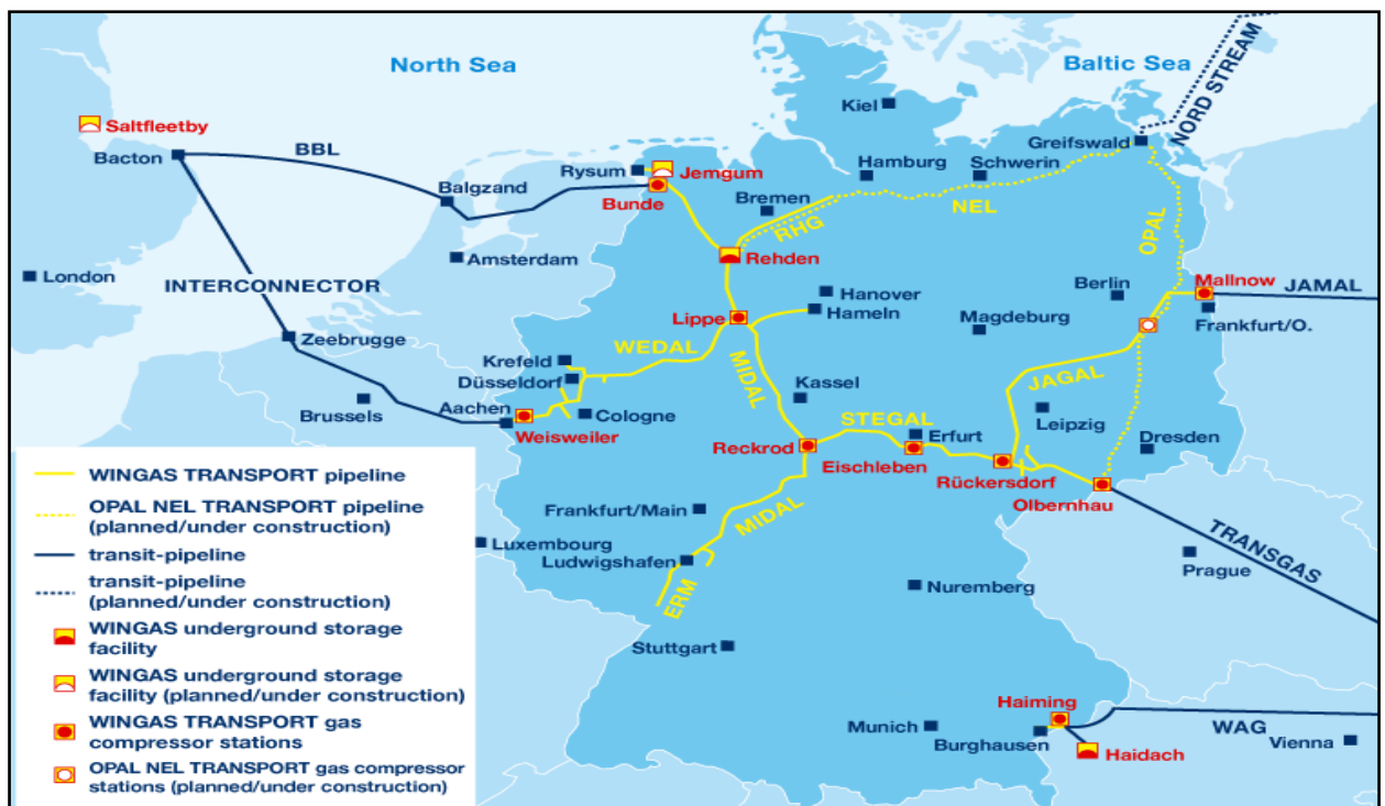
Figure M.3: Onshore connection in Germany: Opal and Nel pipelines
